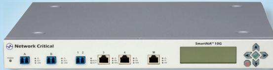
Our revolutionary 10 Gigabit Filtering & Aggregating TAP allows you to TAP into your 10 Gigabit links and then filter and/or aggregate the traffic to meet the needs of your monitoring tools.
